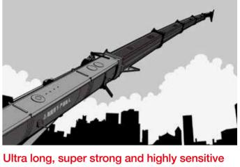
Four-section boom of high strength steel structure and optimized U-shaped cross section reduces weight significantly with higher safety rates. Jib mounting angles are 0°, 15° and 30°, which ensures fast and convenient change-over between different operating conditions so as to improving working efficiency of the
